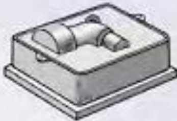
Drag with core set in place
