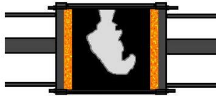
MOLD FOR SLUSH CASTING CROSS SECTIONAL VIEW OF INSIDE OF CASTING A CERTAIN AMOUNT OF TIME ( T_1 ) AFTER POURING
