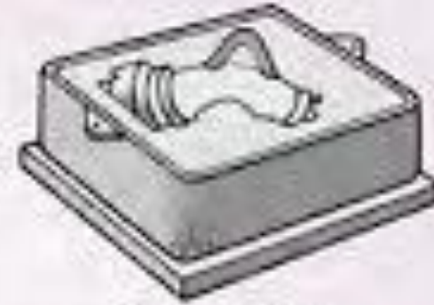
Drag after removing pattern
