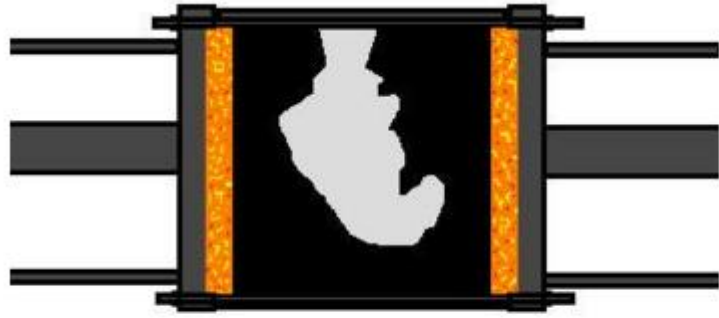
MOLD FOR SLUSH CASTING IMMEDIATELY AFTER POURING
