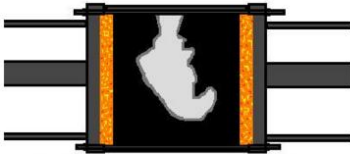
MOLD FOR SLUSH CASTING CROSS SECTIONAL VIEW OF INSIDE OF CASTING A CERTAIN AMOUNT OF TIME ( T_2 ) AFTER POURING ALSO NOTE ( T_2 > T_1 )
