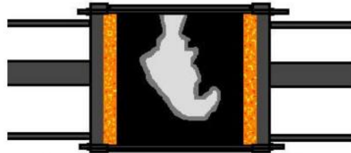
MOLD FOR SLUSH CASTING CROSS SECTIONAL VIEW OF INSIDE OF CASTING A CERTAIN AMOUNT OF TIME ( T_3 ) AFTER POURING ALSO NOTE ( T_3 > T_2 )
