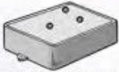
Cope after ramming with sand and removing pattern, sprue, and risers
